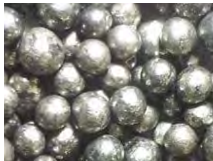
BlastOne's regular shaped, sized and weighted steel shot will give excellent results over and over again.
