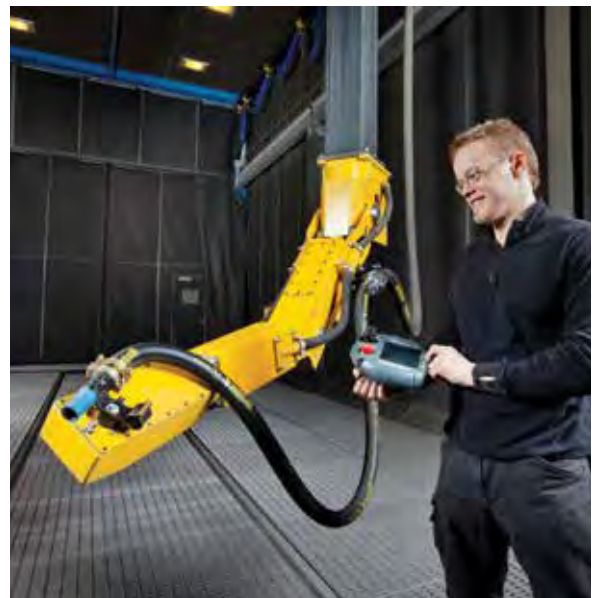
THE ADDITION OF A ROBOT FROM BLASTMAN ROBOTICS CAN TRIPLE PRODUCTIVITY IN BLAST ROOMS
