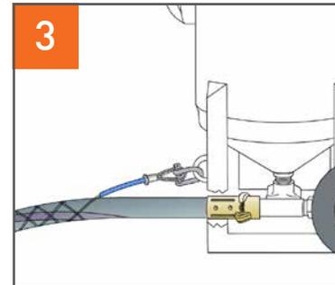
3 Inlet/outlet to blast machine, Air Prep, etc.
