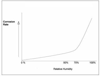
Fig. 2: Corrosion rates vs. relative humidity
