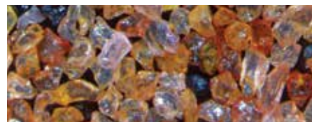
Weak Indian Garnet particles with fracture lines
