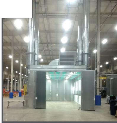
Finished side down draft paint booth with unique paint cure mode for better equipment finishes
